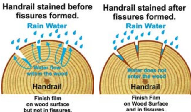
We strongly recommend that handrail be allowed to dry to less than 20% moisture content before doing anything to them. This may take two to six months depending on how green they are and the diameter of the rails.
